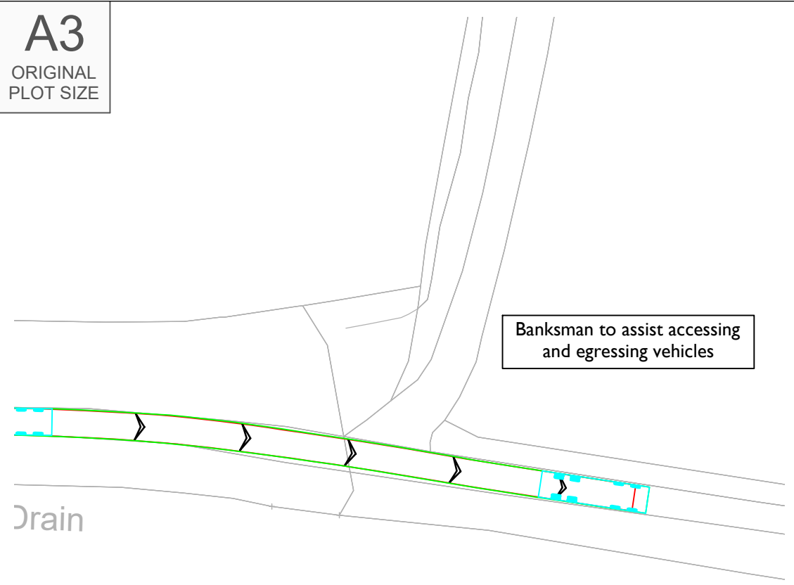
Tipper Vehicle Entering Site
